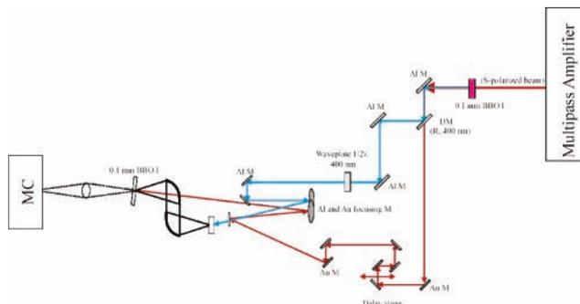
**Figure 7.** Experimental arrangement for femtosecond-domain fluorescence upconversion experiments.
